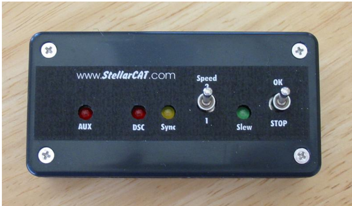
Remote Status Unit showing lights for AUX, DSC, Local Sync, and Slew (permissive). Switches are for Speed 1/2 selection (for wide or narrow FOV's) and an E-Stop switch. Price is $89 + S&H
